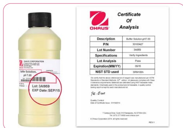
Expiration dates are printed on the label of the buffer bottle, and according to the LOT code visit ohaus.com/Lot-Certificates
